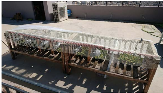
Figure 11 This is the outdoor installation using separators between cases and a cover in order to control quantity of water from rain
