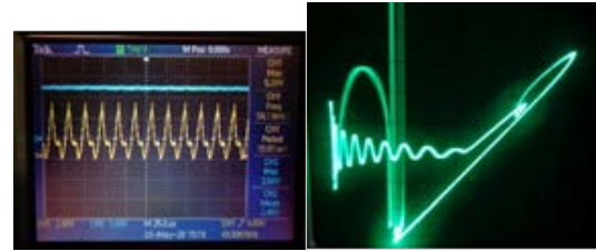
Figure 2 (Left) LED Driver period-1 response, 50 kHz, Time-domain waveform
